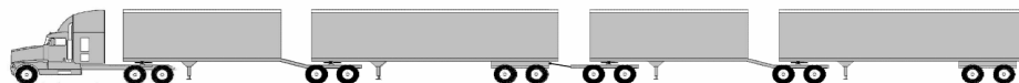
Tractor Semi trailer w. 5th wheel Semi trailer Dolly Semi trailer w. 5th wheel Semi trailer
