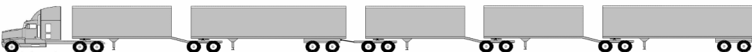
Tractor Semi trailer w. 5th wheel Semi trailer Dolly Semi trailer w. 5th wheel Semi trailer w. 5th wheel Semi trailer
