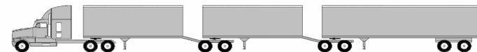
Tractor Semi trailer w. 5th wheel Semi trailer w. 5th wheel Semi trailer
