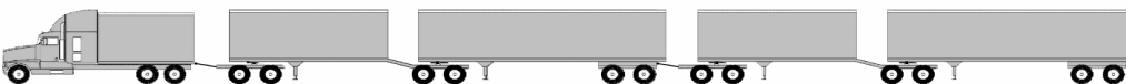
Straight truck Dolly Semi trailer w. 5th wheel Semi trailer Dolly Semi trailer w. 5th wheel Semi trailer
